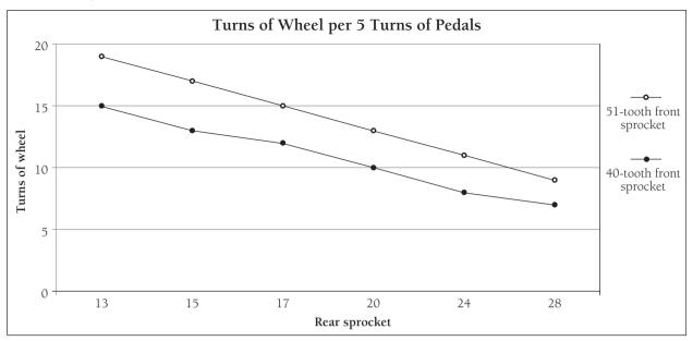
Important note: The horizontal scale is not linear (equal increments). Instead, it represents a typical cluster of gears.
