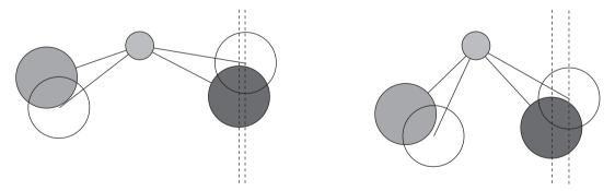
When it tilts, the centre of each weight moves only a small distance, as shown by the vertical lines going through the centre of the black weight and the clear circle representing the position of this weight after tilting. The tightrope walker on the right has its skewers for the grey and black weights at steeper angles. For the same amount of tilt, the centre of each weight moves a larger horizontal distance, represented by the gap between the dotted lines.
