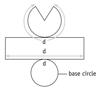
The distance around the outside of the part-circle must match the length of the side strip and the circumference of the base circle. The best way to make this net is to make the part-circle first and use string to measure the other lengths.
